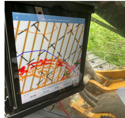
Mistik contractor use of monitors in their harvesting equipment to ensure adherence with the in-block harvest plan.
